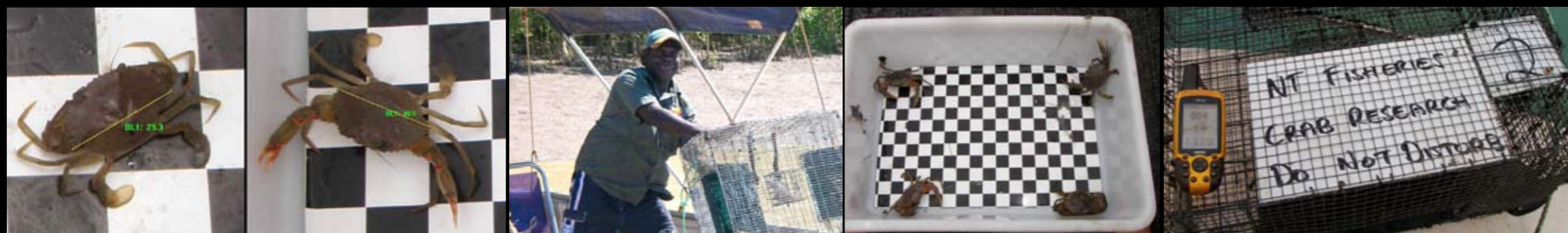
Images from bottom left to right: Juvenile mud crabs being measured using image analysis software, Yugul Mangi ranger Benjamin Wilfred checking research pot, Crabs captured are emptied into a plastic tray which has a checkerboard pattern applied to the inner surface for calibration purposes, Digital image showing individual pot number and GPS readout.
