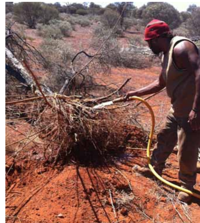
Before weighing the tree all the soil was cleaned off the root system. This was then cut from the stem using a chainsaw.
