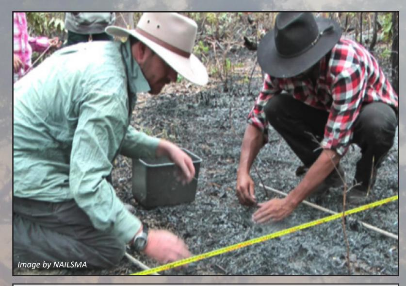
Then they do all the measuring again in the burnt areas. The difference between the 'before burning' and 'after burning' measurements is the amount of fuel that has burnt and become smoke. The smoke contains the greenhouse gases.
